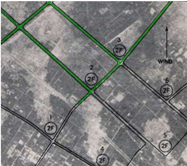
Fig 5. The planning protocol to Allied bombing generated mass-fire. This photo and its overlay constitute a fire susceptibility plan—a reverse fire protection plan, therefore known as a reverse Sanborn map. This fire susceptibility plan was constructed from photographic reconnaissance by professional fire experts.
